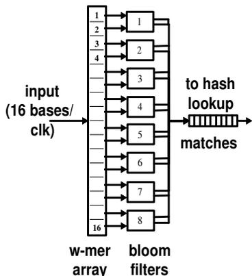
Fig. 5. Bloom filters as used in stage 1a.
