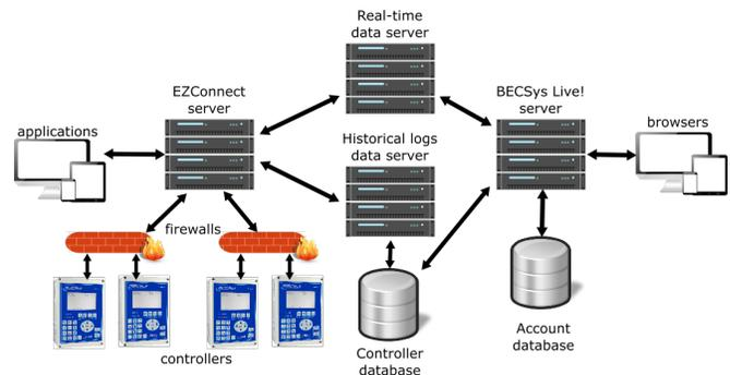
Fig. 1. Aquatic IoT infrastructure. Each of the servers (and databases) are deployed in the cloud and can be replicated to support increased capacity and/or fail-over reliability.
