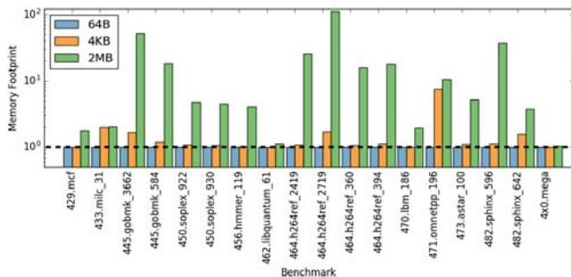
Fig. 4. Memory footprint normalized to 64B granularity.
