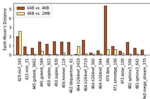
Fig. 5. Comparing (64B, 4KiB) and (4KiB, 2MiB) reuse signatures using Earth Mover's Distance.
