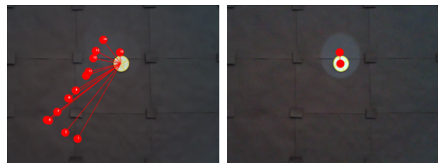
Fig. 13. Control algorithm, sequence of positions (left) and end condition (right).
