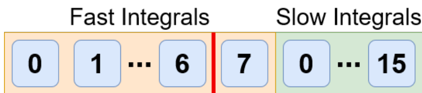
Figure 4.1: Early/late integrals saved in the short and long buffers. To the right of the red line are late integrals; to the left are early integrals.
