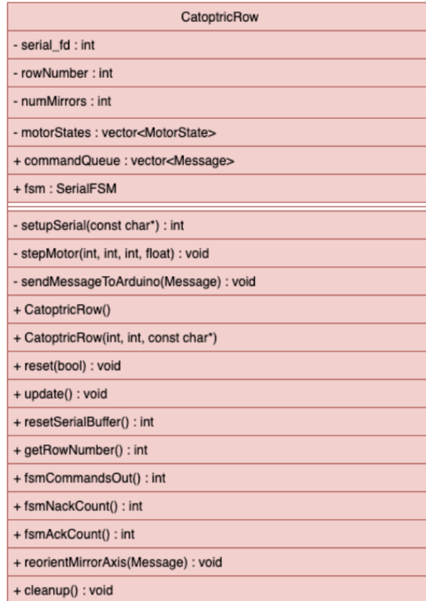
Figure 2.5: CatoptricRow UML diagram.
