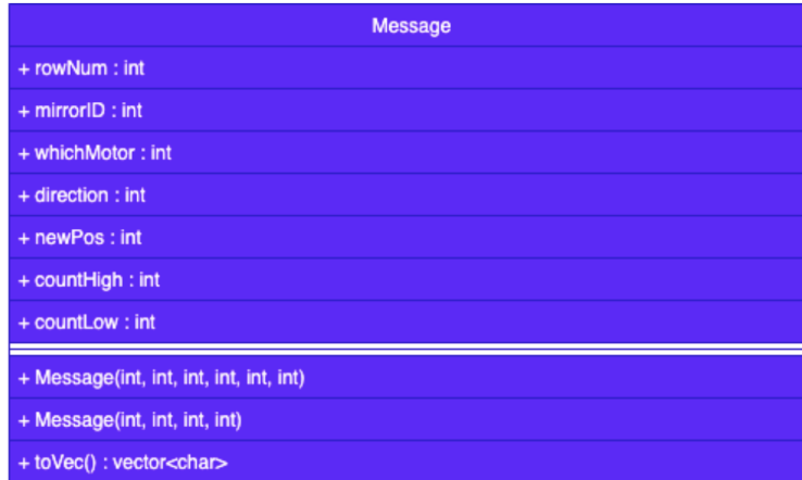
Figure 2.4: Message UML diagram.
