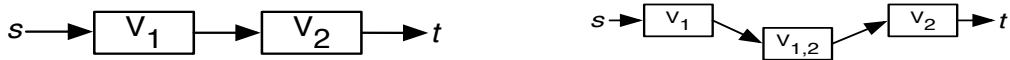
(a) Initial application graph G_A with two compute kernels V_1 and V_2 , a data source s , ( V_{1,2} ) to G_A between compute kernel vertices and a data sink t (b) Addition of a communications vertex V_{1,2} to G_A between compute kernel vertices V_1 and V_2
